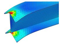
Figure 6.8: Bending illustrated of a vertically loaded thin I-beam (D/t = 40), which shows the top and bottom open end plates turning away and taking less stress: effectively losing their effectiveness.
