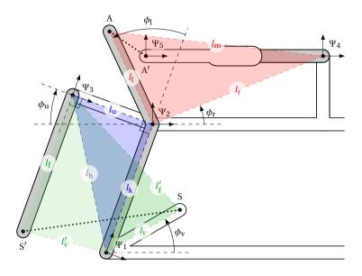
Figure C.1: Full kinematic model of Skippy's hip joint in its zero position (q = 0). The loop closure constraints are not satisfied. Not to scale.
