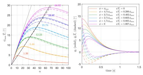
(a) Maximum initial velocity  $\dot{q}_1(0) = \psi_{\text{max}}$ , scaled by (b) Pendulum trajectory as a function of time for var- $T_c$  for comparison with the previous studies that use a jous initial conditions  $q_1(0) = \phi$  and  $\dot{q}_1(0) = \psi$ , with maximum offset angle  $q_1(0) = \phi_{\text{max}}$  instead.
