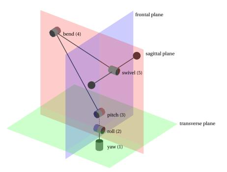
Figure 5.2: A schematic body diagram of Tippy, showing the kinematic tree with joint numbers and names and structural planes. Not to scale. The axes of the second (roll) and third (pitch) joint intersect in reality, but are drawn apart and connected with a dotted line to illustrate their order in the kinematic tree.
