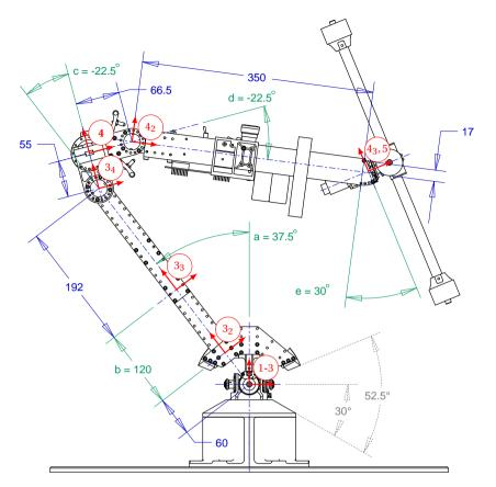
Figure 5.3: Right view of Tippy, scale 1:6.25. Fixed dimensions displayed in blue and tunable dimensions in green with parameters *a* to *e*, with lengths in mm and angles in °. All joint angles are zero (q = 0). Right-handed yz coordinate frames of (sub-)bodies in red, with x pointing out of the drawing.
