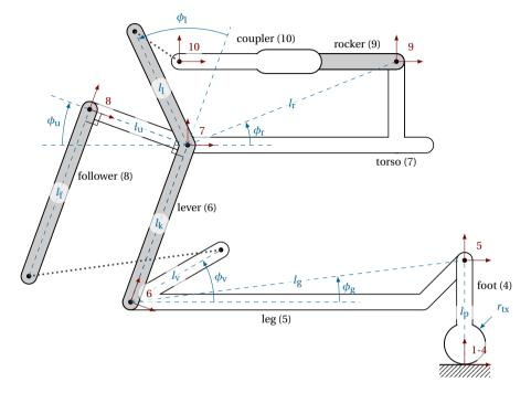
Figure 8.1: Full kinematic model of Skippy in its *open-loop zero* configuration q = 0, not to scale. Loop closure constraints would be satisfied if the points connected by the two dotted lines coincided, forming revolute joints. Joint coordinate frames and corresponding joint numbers are drawn in red; body names and corresponding numbers are written in black. Their transformations and loop closure kinematics are fully defined by the 14 indicated parameters.
