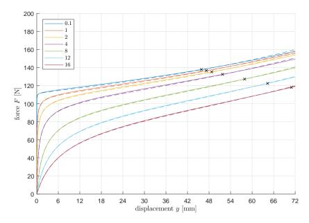
Figure 7.3: Spring profile: force *F* versus displacement *y* according to FEAs (solid) and algebra (dashed) for various arc widths *a* (see legend). Parameters:  $k_c = \pi^2/4$ ,  $\lambda = 0.6$ , L = 144 mm, I = 6.75 mm<sup>4</sup>, E = 35 GPa. Black x-marks correspond to a maximum compressive strain of  $\epsilon_{xc} = 0.21$  according to FEAs, which is assumed to be the compressive strain at which material failure is imminent (see also fig. 7.6).
