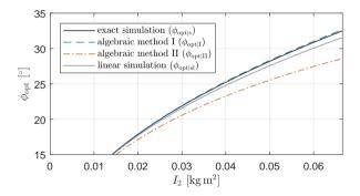
Figure 4.3: Results of algebraic method I ( $\phi_{opt|I}$ ) match very well with those of the exact simulations ( $\phi_{opt|s}$ ) and slightly poorer—but still well—with those of simulations with a linearised component of the gravity force ( $\phi_{opt|sl}$ ). Results of algebraic method II ( $\phi_{opt|I}$ ) match much poorer with both  $\phi_{opt|sl}$  and  $\phi_{opt|sl}$ .
