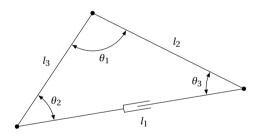
Figure B.1: A simple triangle mechanism that has one edge of variable length  $(l_1)$ , used for calculation of triangle functions  $\gamma_{\tilde{T}}$  and  $\gamma_{\hat{T}}$ .
