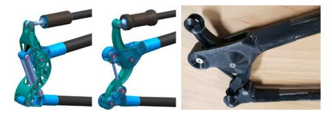
Figure 6.9: The left and centre figure depict Skippy's four-bar linkage in the new and old design style respectively. The right image shows a prototype 3D print of the old design, which was found to be unsatisfactory regarding both manufacturability and performance.
