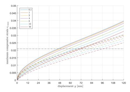
Figure 7.5: Maximum compressive strains corresponding to data in fig. 7.3, with strains according to eq. (7.13) with  $M_b = M$  and  $F_n = F$  dashed. The fit is poor. The failure compressive strain  $\epsilon_{xc} = 0.021$  is plotted dash-dotted in black.
