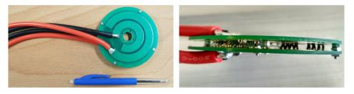
Figure 6.2: The pancake-style slipring that would have been mounted on Skippy if batteries were to be placed in the crossbar.
