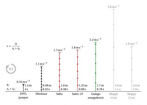
Figure 2.3: Visual representation of the vertical jumping agility v of various jumpers. The graph has been copied from Haldane et al. (2016b), and has been amended with data of Salto-1P (Haldane et al., 2017) and hypothetical data of Skippy if it were jumping 4 m and 2 m high. The number of arrows correspond to the number of repeated jumps over an interval of 4 s, and the length of each arrow is proportional to the jump height *h* of one jump.
