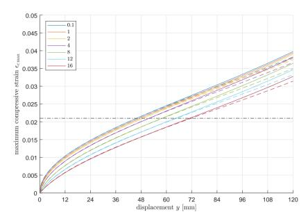
Figure 7.6: Maximum compressive strains, similar to fig. 7.5, but with theoretical values compensated by a shape factor such that  $M_{\rm b} = 1.25M$ .
