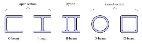
Figure 6.6: Examples of open and closed beam section designs based on which structural components in robots can be designed.
