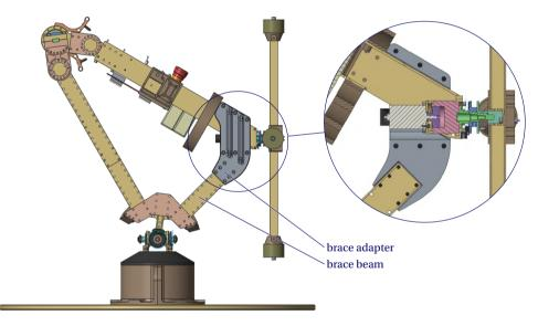
Figure 5.7: Tippy depicted with its brace, consisting of a brace mount and beam, designed and installed to improve its structural stiffness for swivel balancing experiments (in the frontal plane).
