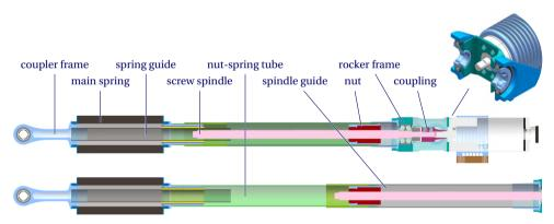
(a) Main actuator using a ball screw, depicted for Skippy fully extended (above) and flexed (below). The actuator length is limited by the guiding arrangement, a light-weight solution to resist buckling and provide ingress protection.
