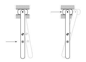
Figure 6.20: A slender beam suspended from a pivot on a frictionless slider, with the CoM (O) at  $c_x = 1/2l$  and the CoPc (O) at  $p_x = 2/3l$  from the pivot point. The initial response is shown in grey: if struck by an impact at the CoPc (left), then no initial displacement occurs at the pivot, and the other way round (right).
