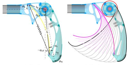
(a) Kinematic triangle of the ankle spring.
