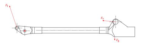
Figure 6.11: Free body diagram of the torso depicting forces as implemented in an FEA. The forces correspond approximately to those of Skippy close to its nadir while preparing its highest hop, which is one of the most demanding scenarios. The red dot is the fixed joint in FEA; its reaction forces are not drawn.
