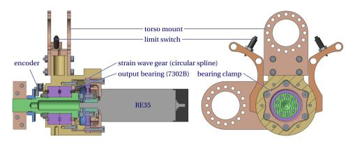
Figure 5.6: Tippy's bend joint actuator assembly, comprising a custom housing for the strain wave gear, strong output bearing, encoder and customizable mounting options for the leg, torso and bend joint end stops with limit switches. This assembly depicts the hip adapter (fig. 5.4h) and hip housing (fig. 5.4i) sub-bodies.
