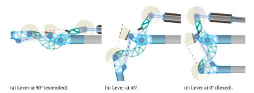
Figure 6.14: Skippy's hip range. The distance between the red dashed lines is the moment arm of the follower  $a_{\rm f}$ . When Skippy is fully flexed (more torque)  $a_{\rm f} = a_{\rm f,flx} = 5\,{\rm cm}$  and when it is fully extended (more speed)  $a_{\rm f} = a_{\rm f,ext} = 2\,{\rm cm}$ .
