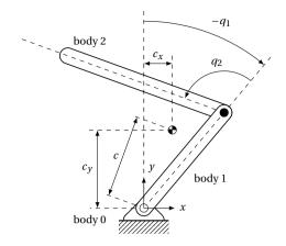
Figure 3.3: The mechanism of a 2R planar balancing machine, where only the second joint is actuated, like the Acrobot.
