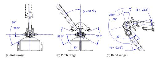
Figure 5.5: Joint ranges as defined by end stops.
