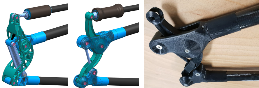
Figure 6.9: The left and centre figure depict Skippy's four-bar linkage in the new and old design style respectively. The right image shows a prototype 3D print of the old design, which was found to be unsatisfactory regarding both manufacturability and performance.
